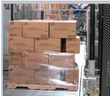
A high speed robotic stretch wrapper in motion, wrapping horizontally from bottom to top.
