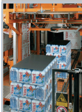
Pallet loads entering a stretch holding system. Here the product is encased in film in one motion from above the pallet, rather than the film wrapping around the sides of the pallet.
