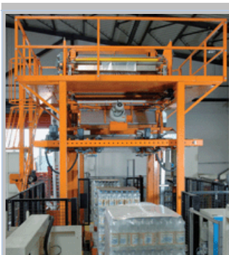
Pallet loads exiting a stretch hooding system. The presealed hoods offer protection from water and any other possible external contaminations.
