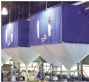
A bulk loaded Gravity system releases loose-fill to the packing stations on-demand
